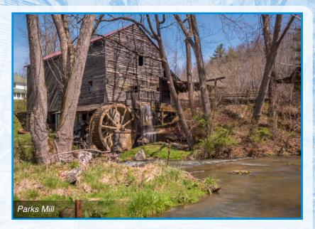
and wheel to generate the flow of water from Fifteen Mile Creek, enabling the water wheel to turn, thus providing power to grind the grain. To date, Parks Mill still has the capability of grinding grits and cornmeal, and has served as a popular attraction for Washington County residents and tourists.
