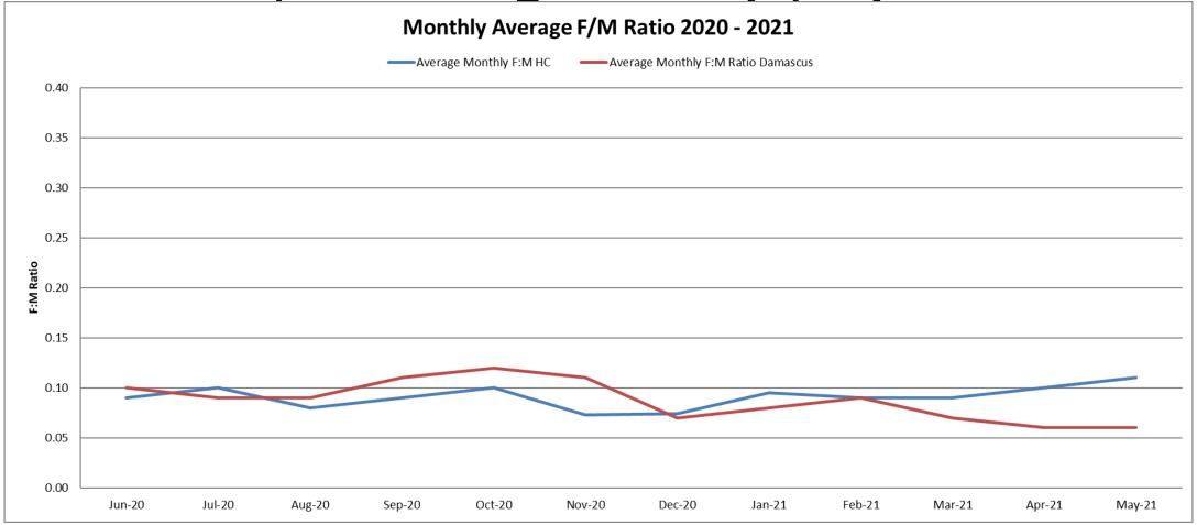
F:M is monitored on a weekly basis as a process control test. This means that the test is not required by DEQ but helps WCSA monitor treatment so that our regulated samples are in compliance.
